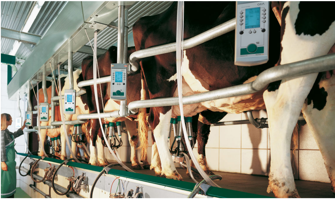
Herringbone parlors are very common in the U.S. Cows stand at an elevated platform that is angled away from the operator in this parlor type.
